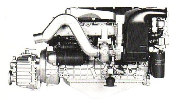
The BMW D 190 W Marine Engine with reversing-type gearbox: 121 kW (165 bhp). Particularly suitable for displacement boats and fast planing cruisers through its compact dimensions and extremely low weight: 60 kg/132 lb less than most of its competitors.
